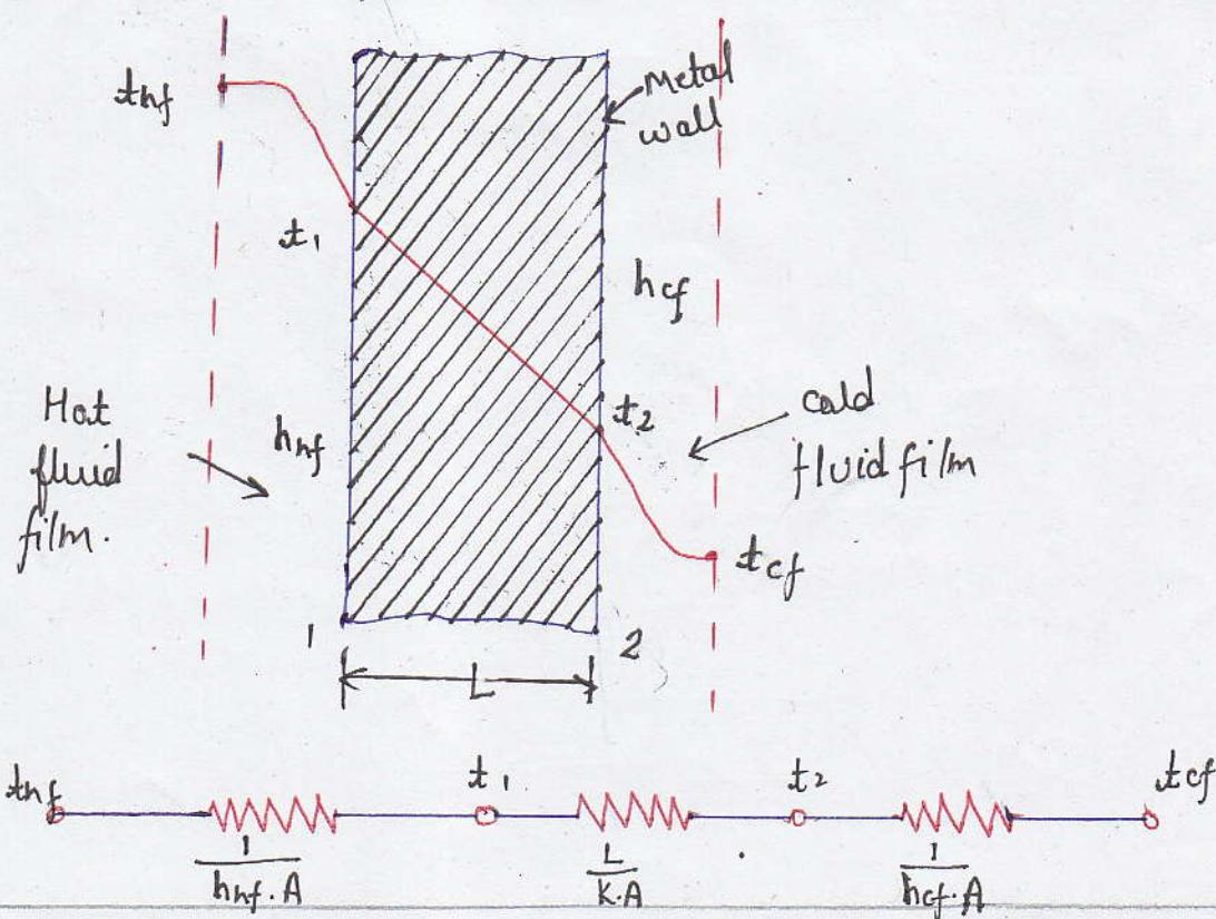
The eqn's of heat flow through the fluid and the metal surface are given by
