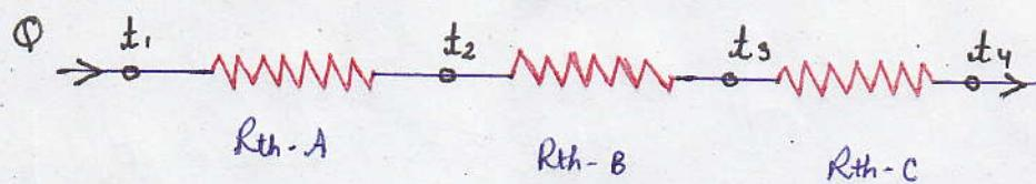
$$R_{th} = \frac{L_A}{k_A \cdot A}, \quad R_{th-B} = \frac{L_B}{k_B \cdot A}, \quad R_{th-C} = \frac{L_C}{k_C \cdot A}$$
